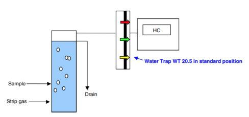
Advantage: In case of a clogged flow, the HC-FID is protected from harmful water
