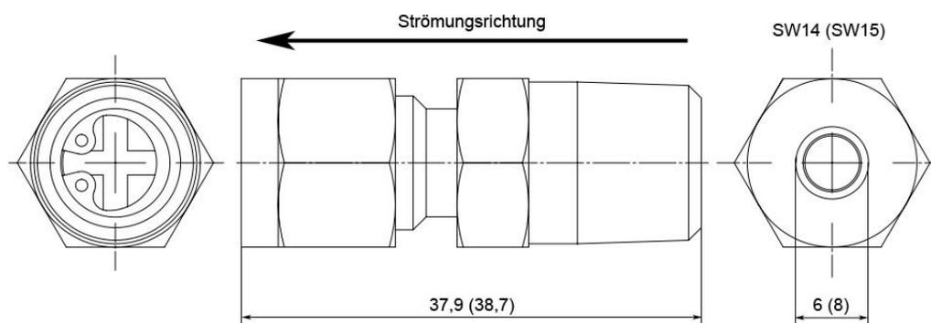
Dimensions (in mm) / values for 8mm tube connection
