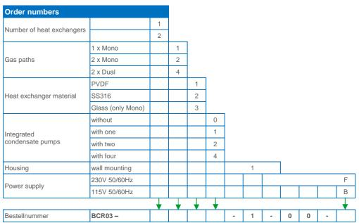
Order example: BCR03-2424-1-00-B → Sample gas compressor cooler BCR03 with 2 dual heat exchangers made of SS316, with 4 integrated condensate pumps, in wall mounting housing and with power supply 115V 50/60Hz
