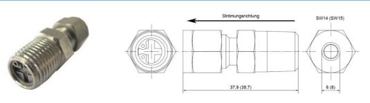
Pressure Reduction Valve – see also PDS PSG PR Part No. 80060195 ( $\varnothing$  = 6 mm), resp. 80060675 ( $\varnothing$  = 8 mm)
