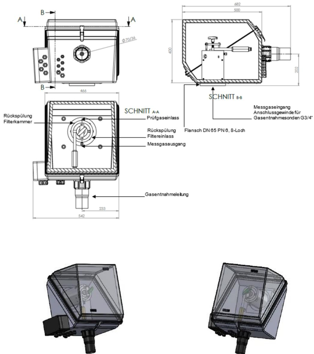
Abmessungen in mm
